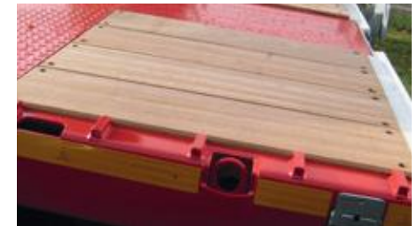
Square iron ledges 20 x 20mm all 200mm of the beavertail of the loading platform.
