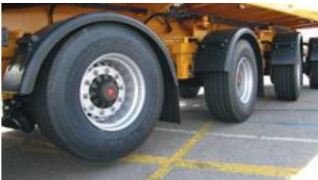
1st axle as liftaxle (depending on the load) lifting with air bag.
