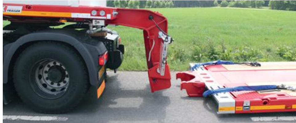
Steel-ramps to bridge the deck hooks
