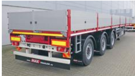
Alu-sideboards in the loading area, height \pm 600 mm, with foldable KINNEGRIP stakes.
