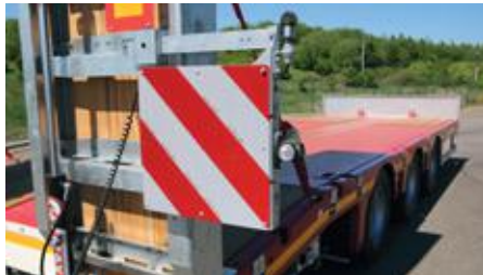
Warning boards ca. 423 x 423mm extendable by 400mm with 1 LED position lights.
