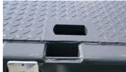
WADER containerpockets in the loading platform for one 20" container.
