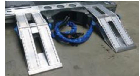
ALU ramps VFR 120 to bridge the deck hooks
