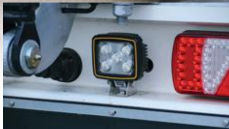
LED working lamps at the rear of the trailer.
