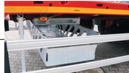
Galvanised storage under the loading platform (2,430 x 770 x 400mm).
