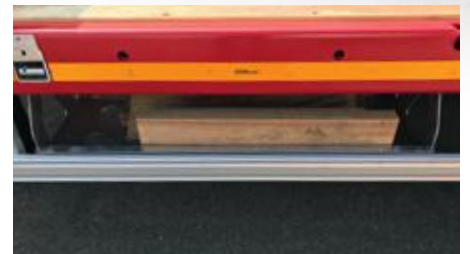
Galvanized storage for timber left and right under the loading platform.
