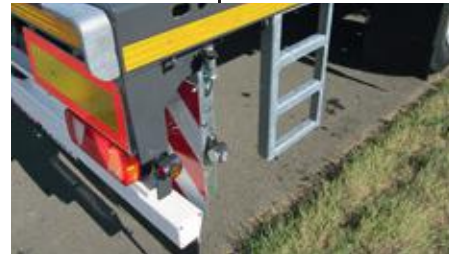
Ladder mounted on the left and/of right hand side.
