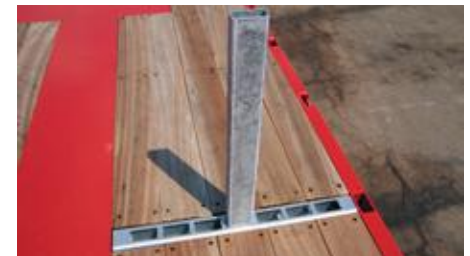
Rows of stake pockets in the loading platform for stakes 100 x 50mm.
