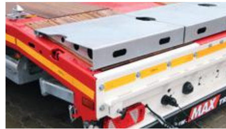
Compensating wedge galvanized for chamfer 1,000 x 8°.
