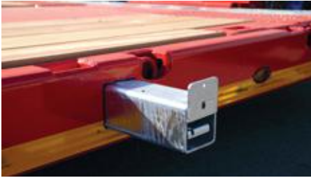
Galvanised outriggers, extendable up to ca. 230mm per side.
