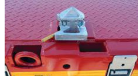
Pockets for stakes ca. 100 x 50mm in the outer frame of the loading platform.
