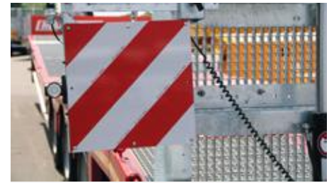
On the right and left under the gooseneck and at the ramps of the trailer one holder for the warning boards and socket.
