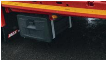
One lockable tool-box HDPE 620 x 360 x 610 / 1,200 x 500 x 480mm.
