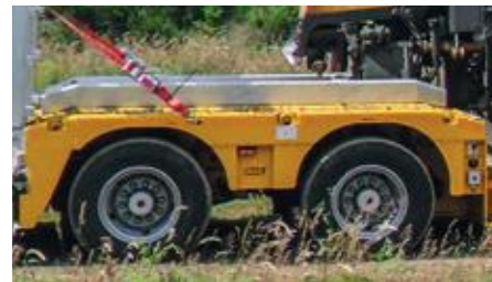
Guidance rails chamfered at the rear to insert on the bogie for chain machines.
