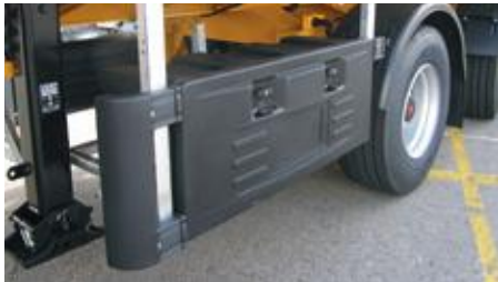
One lockable tool-box HDPE 1,200 x 500 x 480 under the loading platform
