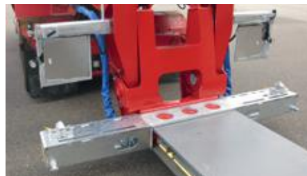
One removable (galvanised) sliding bolste for 1 pairs of WADER containerpockets. WADER-containerlocks.
