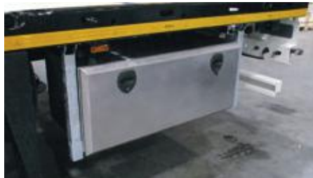
One lockable tool-box INOX 1,200 x 460 x 550 under the loading platform.
