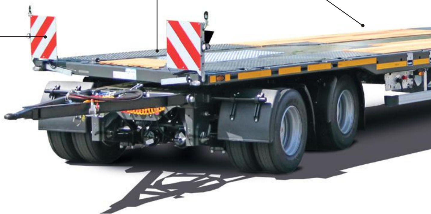
WADER containerpockets in the loading platform for one 20" container.
