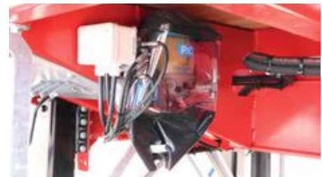
Central greasing BEKAMAX (Pico) with NLGI-2 normal grease with removable protection around the pump. (Only MAX210)
