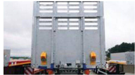
A galvanised steel headboard, height ca. 2,200mm.
