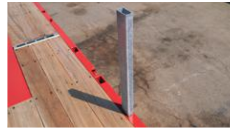
Pockets for stakes ca. 100 x 50mm in the outer frame of the loading platform. Galvanised stakes ca. 100 x 50mm, height 1,000mm.
