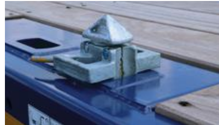
WADER containerpockets incorporated into the loading platform.
