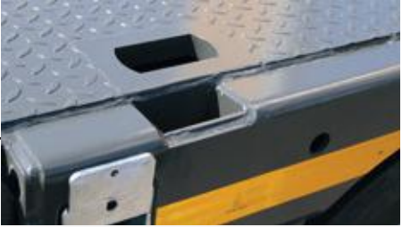
Pockets for stakes ca. 100 x 50mm in the outer frame of the loading platform.
