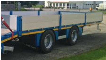
Foldable Alu-sideboards in the loading area, height \pm 400 mm.
