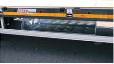
Galvanised storage for timber left under the loading platform.
