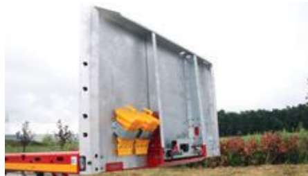
A galvanised steel headboard, height ca. 1,200mm.
