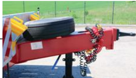
A +/- 1,750mm long drawbar, with a drawbar eye (50mm, 57mm or 68mm diameter).
