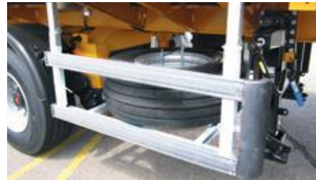
A spare wheel carrier, under the loading platform.
