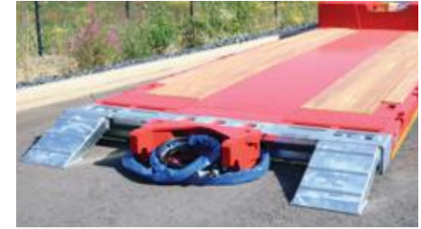
Steel-ramps to bridge the deck hooks
