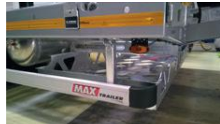
Galvanized storage under the loading platform (2,410 x 1,025mm).
