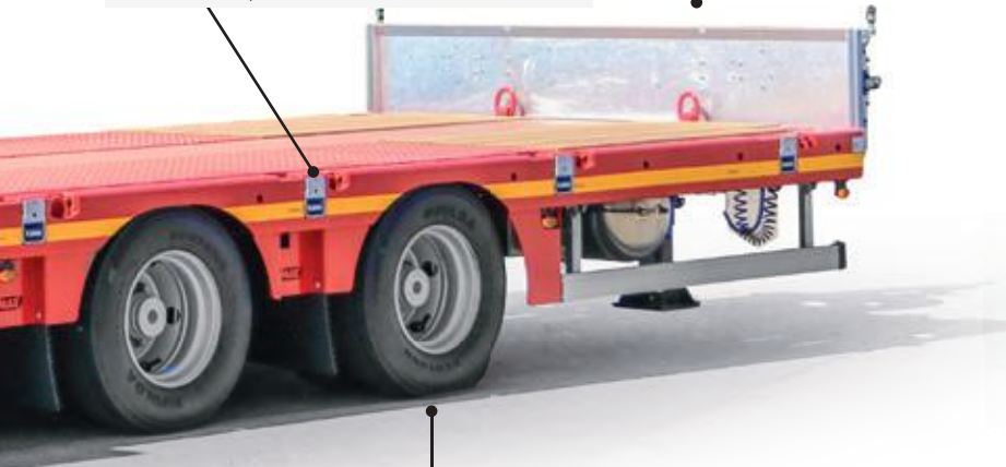
Galvanized outriggers, extendable up to ca. 230mm per side.
