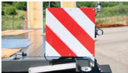
warning boards ca. 423 x 423mm extendable by 400mm with 1 LED position lights
