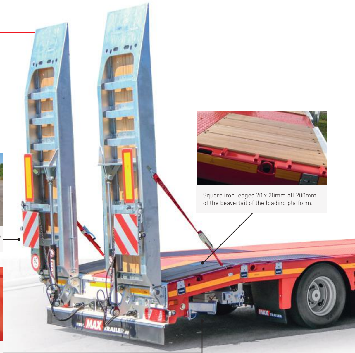
Warning boards ca. 423 x 423mm extendable by 400mm with 1 LED position lights.
