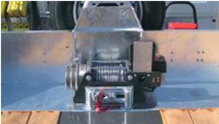
Electric winch with remote control for ca. 5,400kg lifting force included one wire cable diameter 9.5mm length 24m.
