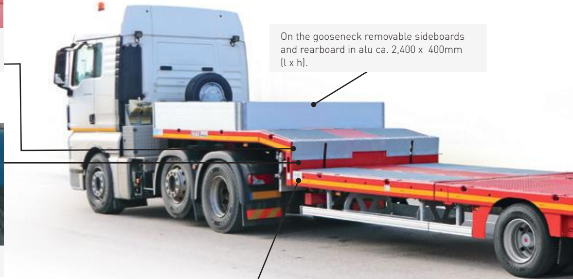
U-beam for ALU-ramps on the rear of the gooseneck with integrated fender.
