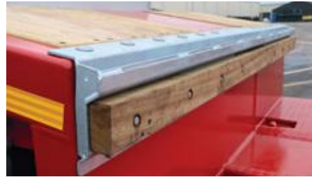
U-beam for ALU-ramps on the rear of the gooseneck with integrated fender.
