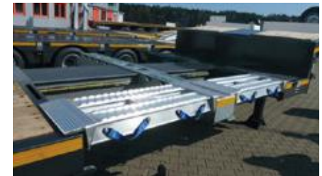
ALU-deck filling sections ca. 1,160 x 420 x 120mm (for an extension of 1,000mm).
