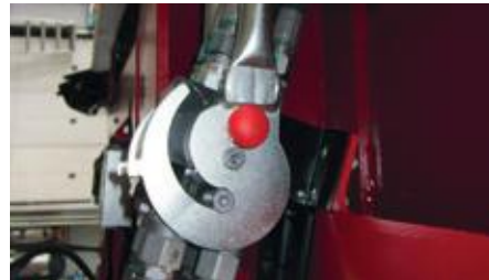
Hydraulic connections from loading platform to gooseneck via multi-coupling insted of screwcoupling. Without guarantee.
