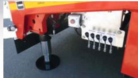
Hydraulic landing gears at rear under the loading platform to increase the loading stability.
