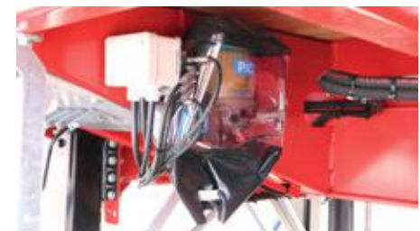
Central greasing with 2 pumps BEKAMAX (Pico) with NLGI-2 normal grease with removable protection around the pump.
