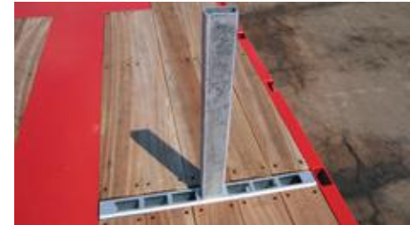
Rows of stake pockets in the loading platform.
