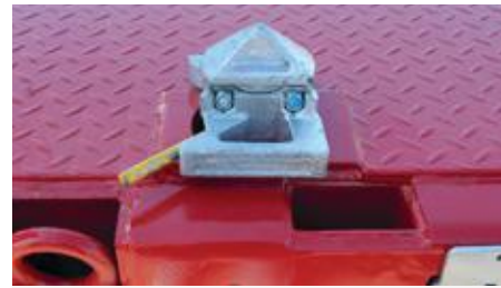
WADER containerpockets in the loading platform for one 20' container. WADER containerlocks.
