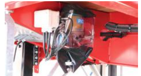
Central greasing BEKAMAX (Pico) with NLGI-2 normal grease with removable protection around the pump.
