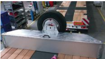
Toolbox galvanized integrated into chamfered gooseneck
